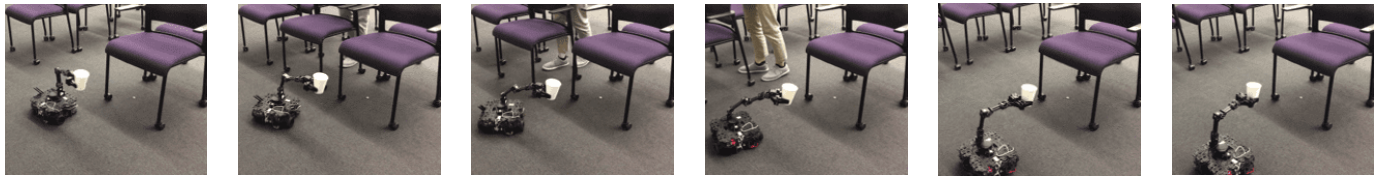
(c) Experimental result with mobile manipulator performing collision avoidance while keeping the end-effector position in the Cartesian space.
